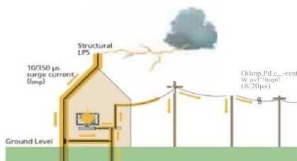
Figure 3: Illustration of lightning current flow from a direct strike to a structure (Source S1)
