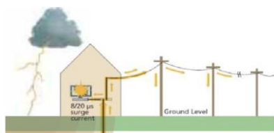
Figure 5: Illustration of lightning current flow from a direct strike near the structure (Source S2)
